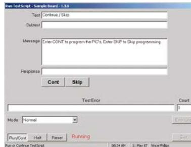
TestWare supports barcode readers so serial numbers and other information about the UUT may be captured at start of a test and stored along with the test results.
