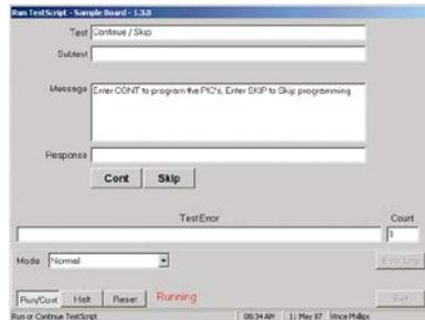
For each test to be run, a test screen similar to the one above is defined. The screen definition is accomplished by dragging screen components onto the screen and defining them.
